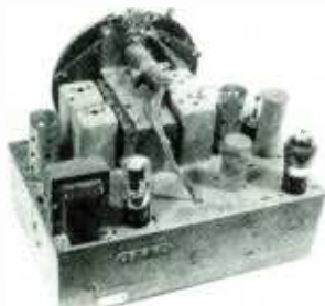
A view of the chassis looking towards the rear of the dial assembly. The horizontal cylindrical unit at the top is the magic-eye tuning indicator.
