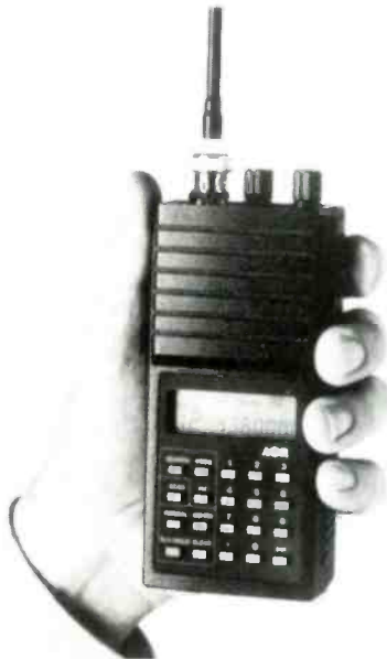
The AR800 handheld scanner covers the 800-MHz band (where the cellular telephones live), as well as a hefty swath of other frequencies (30 to 50 MHz, 118 to 136 MHz, 140 to 174 MHz, 436 to 174 MHz, 436 to 512 MHz and 830 to 950 MHz), providing 20-channel coverage of police, fire, business, industrial, maritime, land/air transportation, and emergency services.
