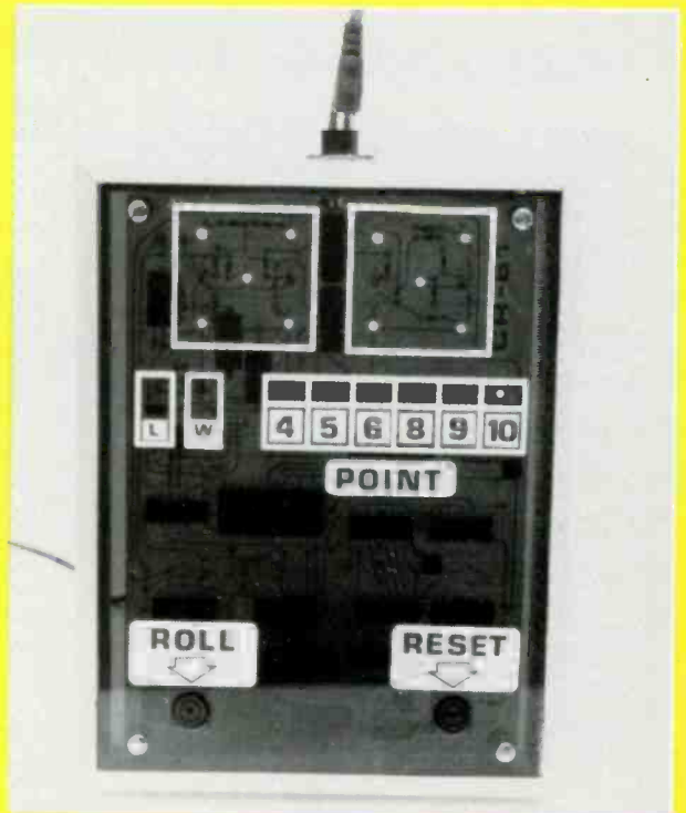
The casino dice game is shown here fully assembled in a wood-frame enclosure. The front panel is laid out in such a way that the boxes (representing the outline of the dice) are positioned just above dice spot LEDs; the "win-lose" boxes ("L" and "W") above LED15 and LED16, and the "point" boxes are over the POINT lamps.
