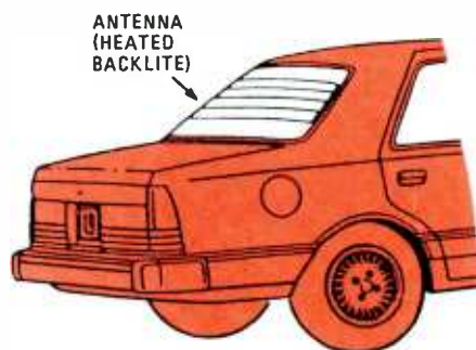
Fig. 13—The HBA is a long-wire design capable of receiving a broad frequency range. It consists of the back-window heater elements designed to allow connection to an amplifier module mounted in a vertical pillar.
